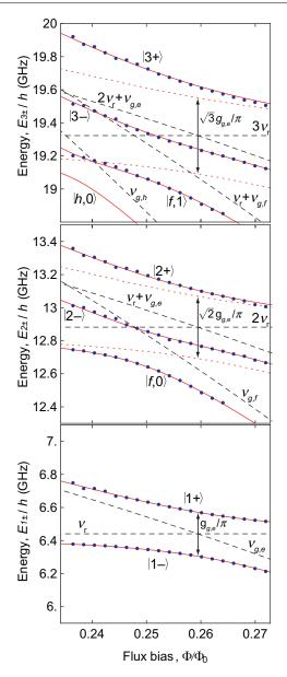
**Figure 5.** Measured energy level diagram of the three-photon/artificial atom system. Measured dressed state energies (blue dots) reconstructed from extracted transition frequencies from data in figure 4 compared to calculated uncoupled cavity and qubit levels (dashed black lines), calculated dressed state energies in the qubit two-level approximation (dotted red lines) and the corresponding calculation including four qubit levels (solid red lines).
